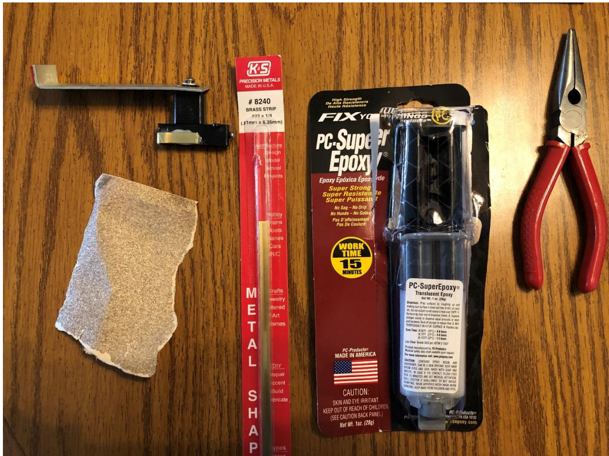
Figure 2 Showing parts and tools required and a repaired adapter
