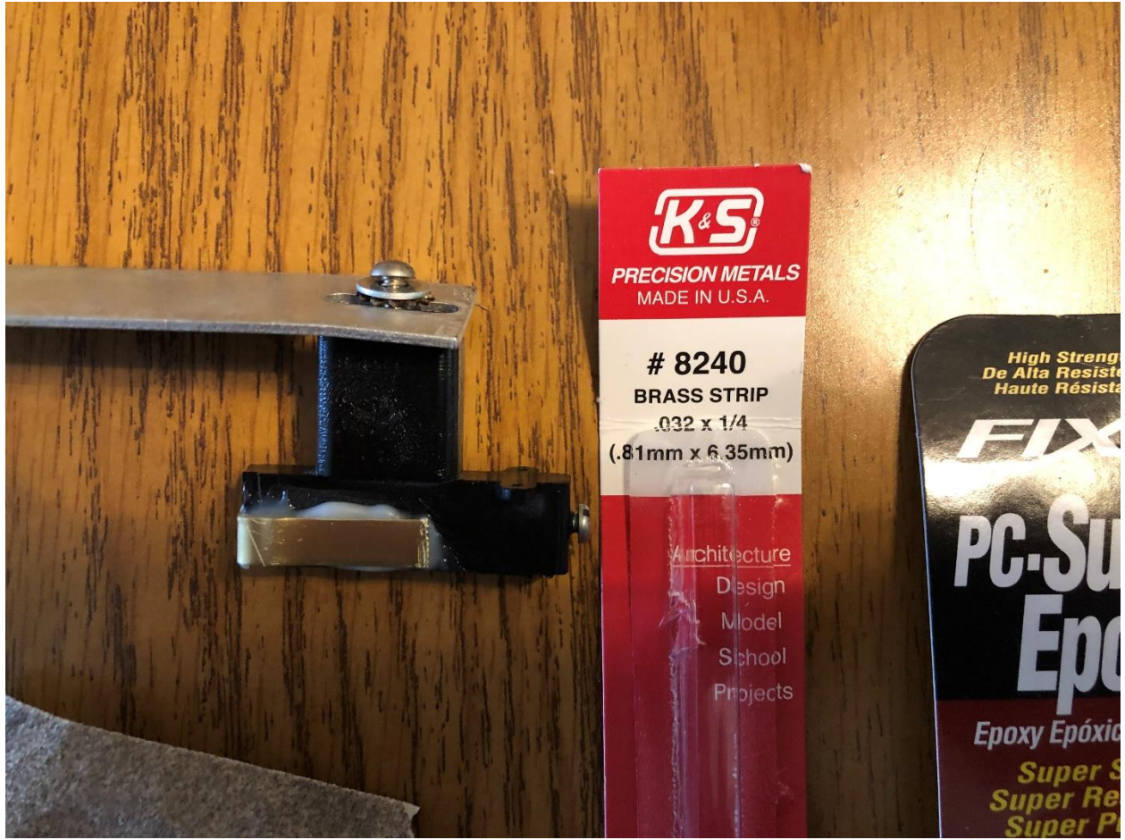
Figure 3 Close up view of repaired adapter and the part number of the brass strip
